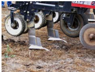
Subsoil ripper/tiller for leaving residue intact
