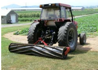
Roller-Crimper for mechanically killing cover crops -
