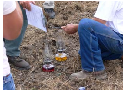
Farmer Ian Heatwole demonstrates petrodiesel fuel vs. clean-burning biodiesel, which he runs in his tractors and pumps. He says there is no difference in performance, but the biodiesel lamp remained clean.
